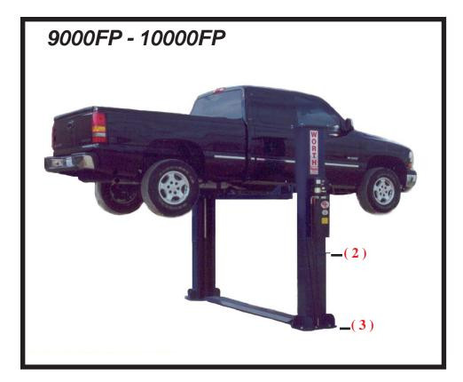
(3) Oversized Base Plates And Gussets - All Worth lifts feature oversized base plates with oversized gussets. Base plates through the model 12000CF are based on a 24"x24"x5/8" minimum size to prevent concrete breakout and offer increased stability.
