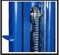
**Dual Chain-Over Hydraulic** cylinders provide superior lifting power and lastability. On average they last twice as long as direct pull or push type cylinders, since the seals only have to travel half as far each time the lift is used.
