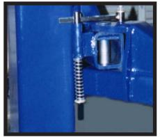
Automatic Arm Restraints lock as soon as the lift begins upward to help prevent load shifting while the vehicle travels up and down. Once vehicle is completely lowered arms release automatically.
